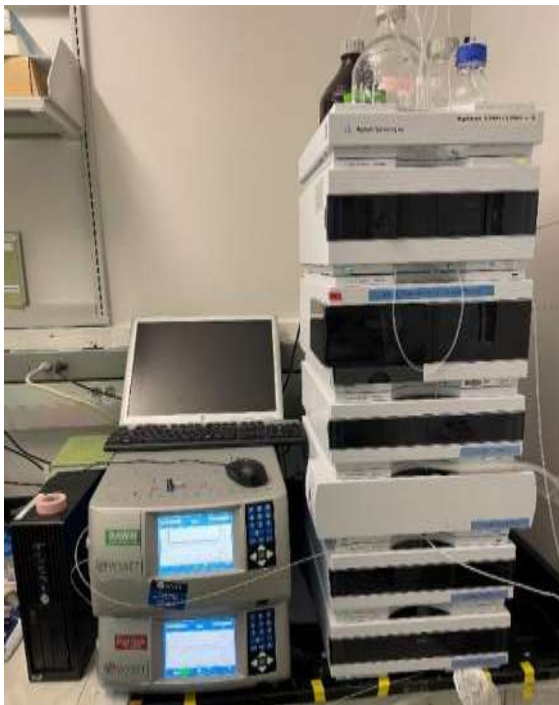
Size exclusion chromatography set up with different detectors
